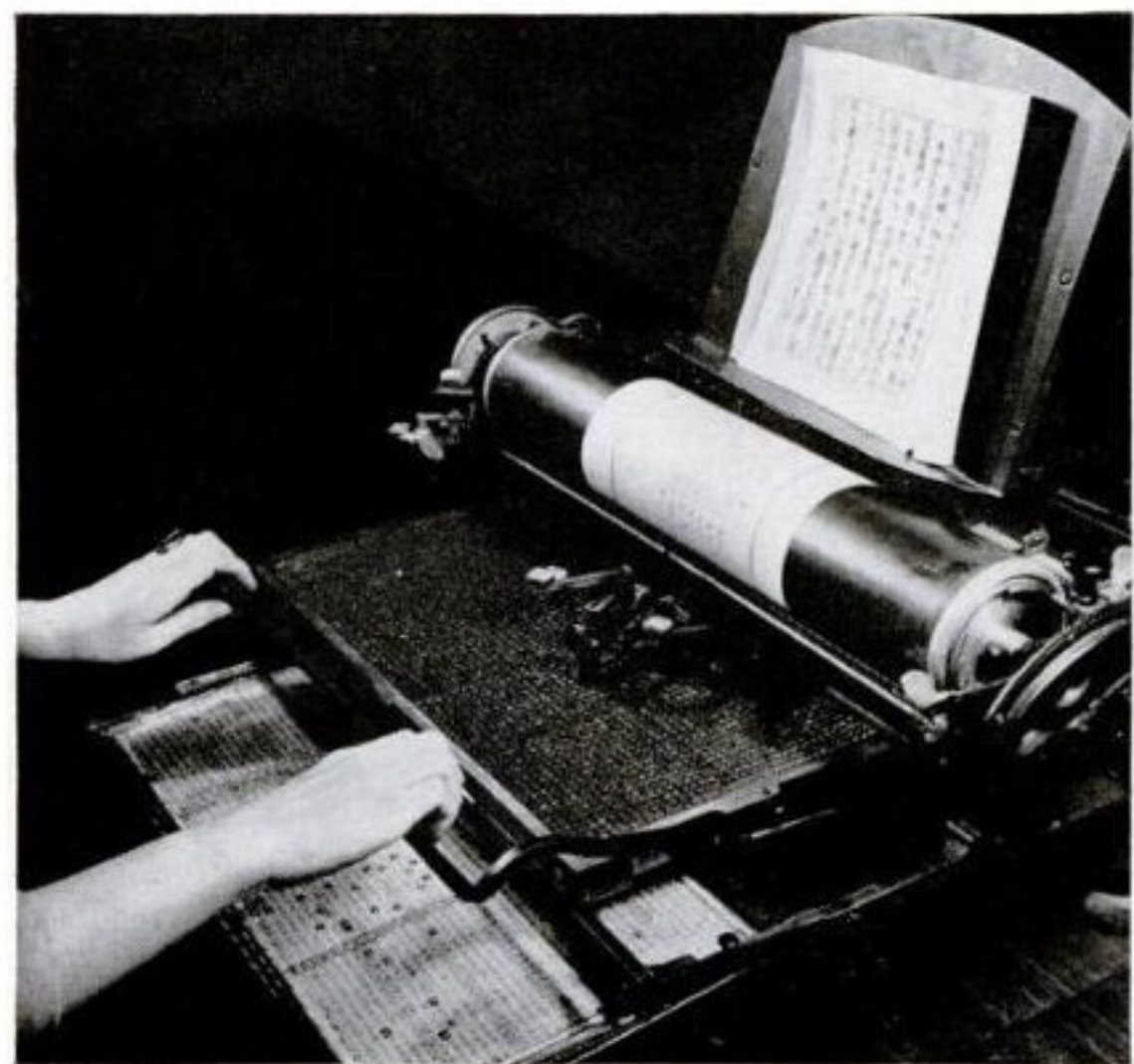
Japanese typewriter , really a miniature typesetting machine with 2,450 characters, yet it types only simplified Japanese. This machine at the OWI is one of 30 in the U. S.
