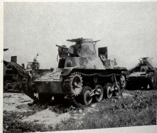
PHOTO 80 Strafing attack set fire to camouflage nets used by the Japanese to conceal these tanks. The fire badly damaged the guns and interior of the tank in the foreground.
