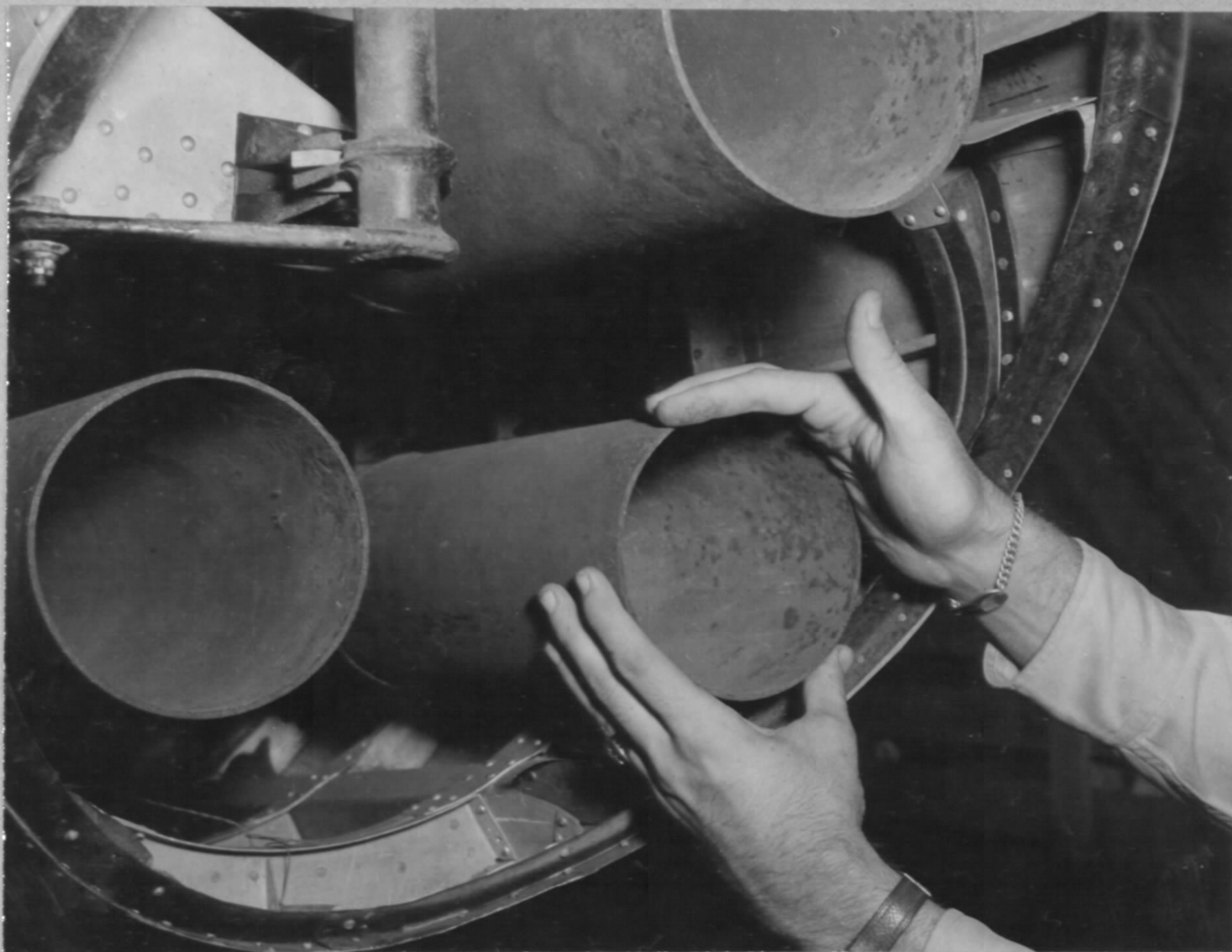
INDEXED Closeup of tail assembly of Jap "Bukabomb". Note the position for three rockets. JAPAN, Sept. 1945.
